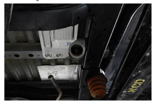
Work the tailpipe over the rear axle, and slide the expanded inlet of the tailpipe over the muffler outlet.
