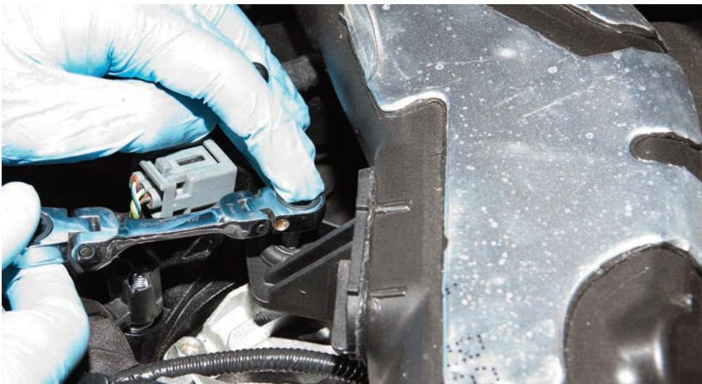
**STEP 3:** Undo the jubilee clips holding the crossover in place at either end of the standard duct
