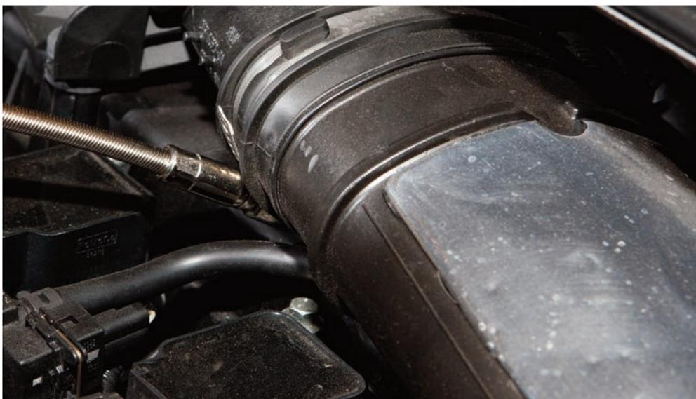
**STEP 4:** With the lower hose removed, pull the standard crossover free from the top hose
