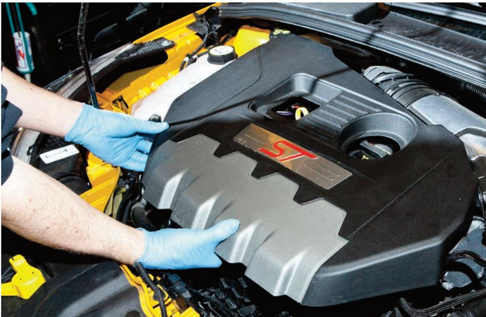
**STEP 2:** Undo the bolt securing the standard crossover duct in-situ with the cam cover
