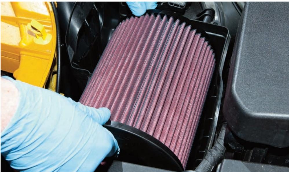
**STEP 8:** Re-connect the convoluted hose between the airbox and the new LLC
