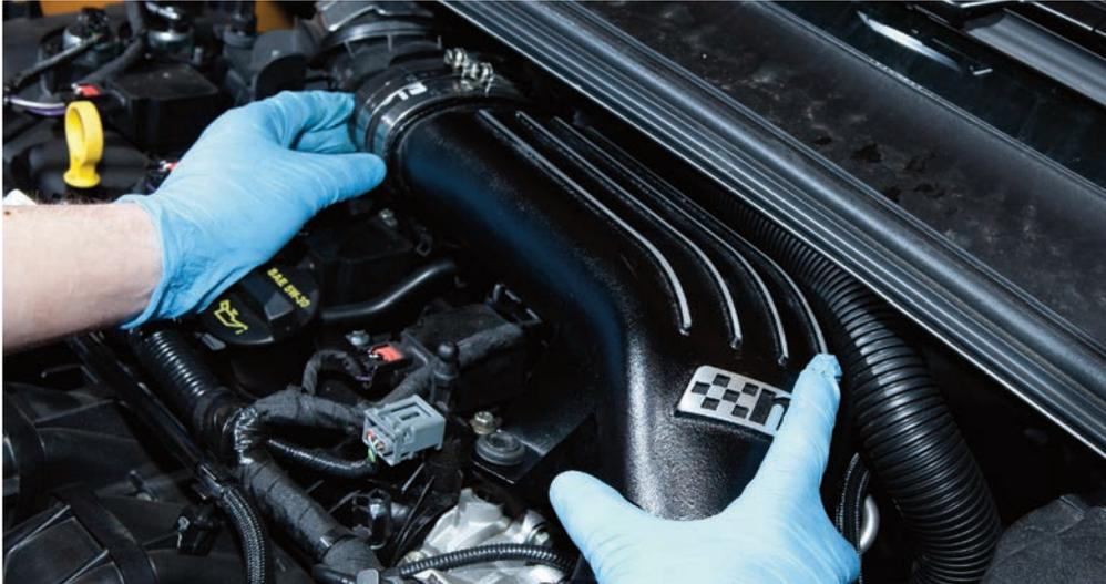
**STEP 7:** Remove the airbox lid by undoing the 4 retaining screws, then replace the standard filter element with the new K&N 57S filter - a detachable plug is supplied with the filter should you require this for homolagation, **optimum performance is achieved wih the plug removed**
