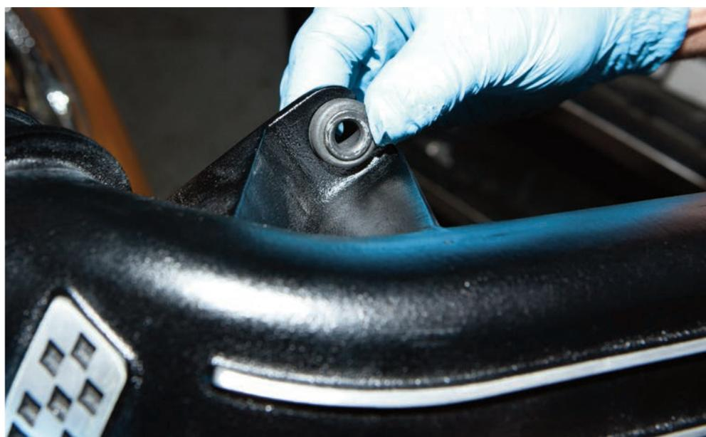
**STEP 6:** Your new crossover is supplied with a silicone hose and clips, make sure the clips are arranged in the orientation shown to avoid fouling
