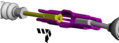
6. Disconnect both parking brake actuation lever cables. **NOTE:** *RH side shown, LH side similar.*
