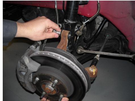
**STEP 8:** While supporting the spindle/rotor/caliper assembly, gently slide the spindle away from the lower strut.
