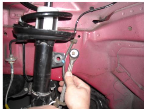
**STEP 5:** Remove ABS wire from the strut housing by gently pulling grogmet from slot.
