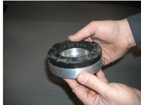
**STEP 17:** Install the new upper bearing assembly onto the new front strut assembly. Install the center insert.
