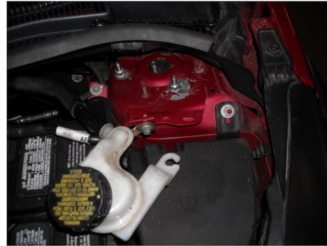
**STEP 10:** While supporting the strut assembly, remove the (3) upper strut bearing retaining nuts and remove the strut assembly from the vehicle. Discard nuts.
