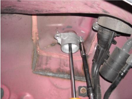
**STEP 28:** Looking at the new upper shock mount, verify the locating holes that are offset face the centerline of vehicle, then place the new coil over assembly into the vehicle.
