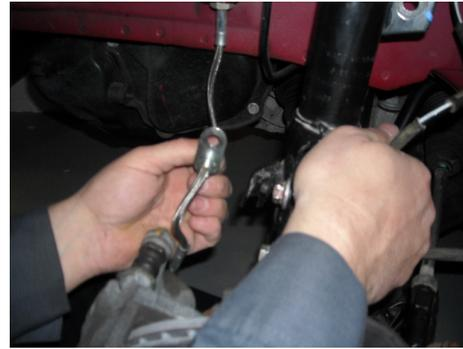
**STEP 7:** Remove the (2) strut to spindle pinch bolts. Discard bolts and nuts.
