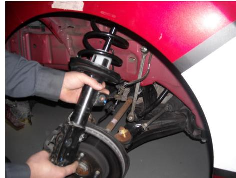
**STEP 11:** Using a spring compression tool, compress the spring and remove the strut bearing center nut. Remove the upper strut bearing assembly.
