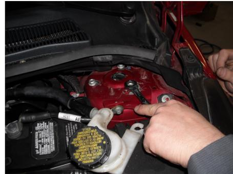
**STEP 20:** Install the brake fluid reservoir onto the locating studs and torque to (62 lb-in).
