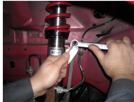
**STEP 23:** Install the front brake line retaining bolt and torque to (19 lb-ft).
