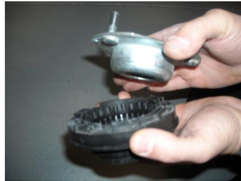
**STEP 13:** Gently pry apart the two halves of the bearing assembly to expose the bearing and race.
