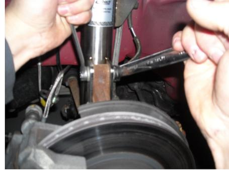
**STEP 22:** Install the front sway bar link into the strut, reinstall the nut and torque to (41 lb-ft).
