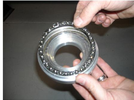
**STEP 16:** Install the upper half of the original bearing assembly onto the new lower half. Verify the upper race is still in its proper placement.
