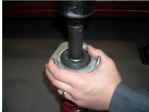
**STEP 19:** Install the strut assembly into the vehicle, install the (3) upper strut bearing retaining nuts and torque to (22 lb-ft).
