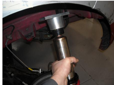
**STEP 29:** Install the (2) upper rear shock retaining bolts and torque to (18 lb-ft).
