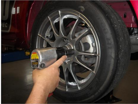
**⚠ WARNING:** Retighten wheel nuts within 160 km (100 mi) after a wheel is reinstalled. Wheels can loosen after initial tightening. Failure to follow this instruction may result in serious injury to vehicle occupant(s).
