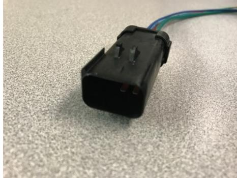
The 6-way pigtail is to be connected according to the chart below. See also the diagrams on the following pages for illustrations of wire connection points, based on the ignition/starter switches that you intend to use. Setup A uses separate toggle switches for ignition and starter inputs, while Setup B uses an ignition cylinder with a key.
