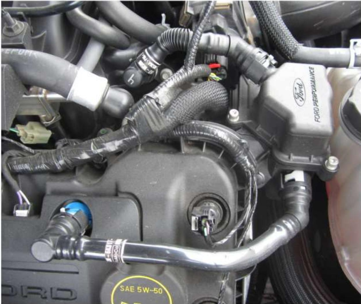
**Maintenance is based on the type of driving the vehicle is subjected to. Track type driving will require more frequent checks for accumulation of oil in the separator. Remove separator and tilt so to empty oil out from the lower fitting. Do not empty from upper fitting! If removal of the top cover is required, when reinstalling, torque socket head screws to 4.5 to 5 Nm.**
