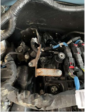
Locate the two bolt bosses indicated in the illustration above. Attach the RH bracket to these bosses using (2) W714962-S437 bolts and torque to 10 Nm (88lbin).
