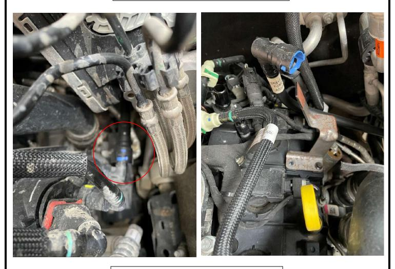
Install LH bracket using (2) W506856-S439 thread-forming screws and torque to 8.5Nm (75lbin). TIGHTEN BY HAND ONLY, DO NOT USE PNEUMATIC OR ELECTRIC TOOLS.
