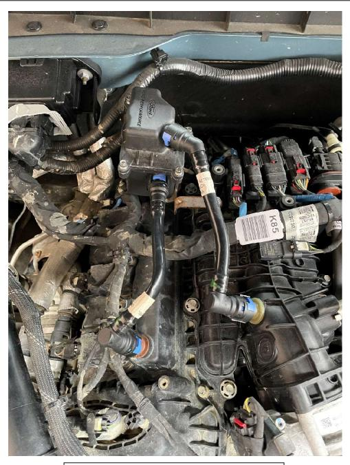
Firmly slide oil separator onto bracket tab. Lubricate inside of PCV connectors with thin film of oil and snap onto camcover, oil separator, and induction tube spigots. Make sure to install completely, looking for blue tab on connector to be locked.
