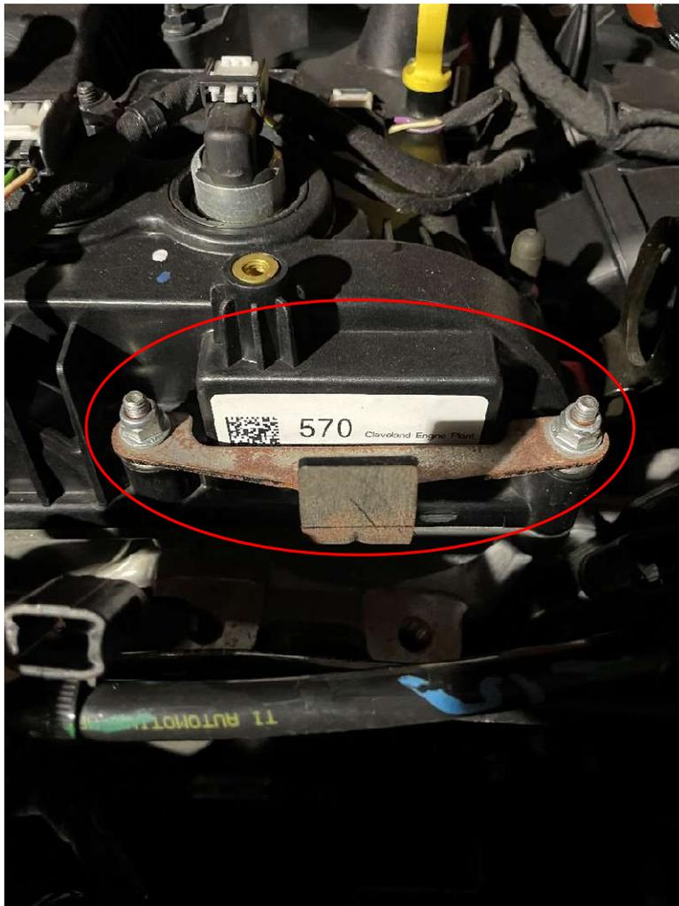
**Remove vacuum line retainers from camcover studbolts, then install bracket over camcover studbolts and install (2) nuts. Torque to 10nm (88lbin).**
