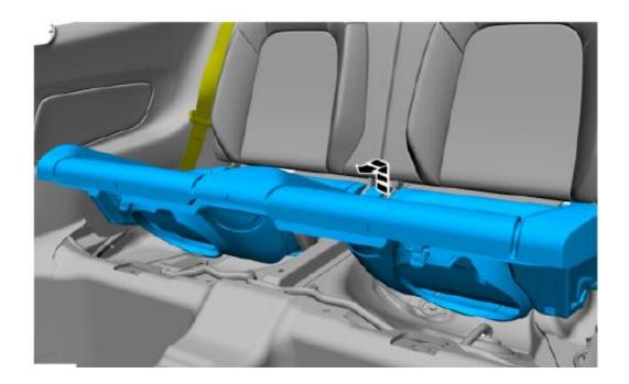
4. LH seat shown, RH seat similar. Remove the nut attaching the seat backrest to the floor.
