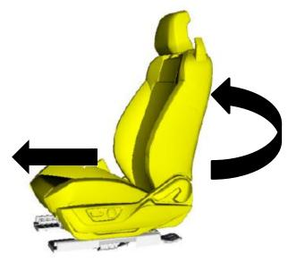
2. The seat cushion tabs must be pressed in to release them from the floor. If the locking tabs are not pressed in, it may result in damage to the tabs.
