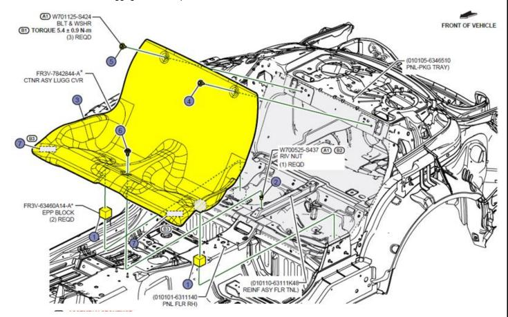
1. Install 2 Foam blocks - Remove release paper and stick blocks in place on floor
