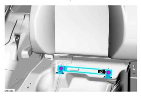
9. Remove the bolt and the safety belt buckle. RH shown, LH similar.
