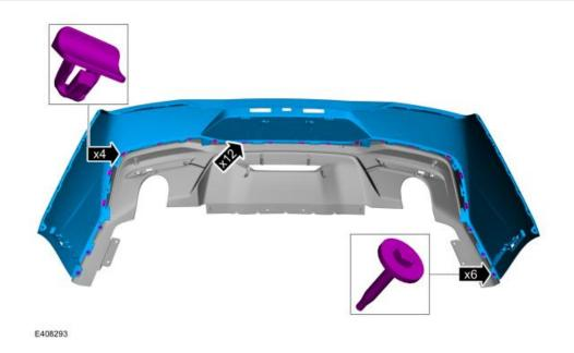
16. install the provided valence by snapping together clips and reinstalling bolts from step 15
