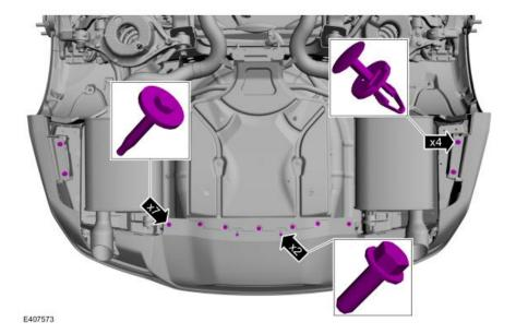
On both sides.Remove the screw, the push pins and position the wheel liner aside.
