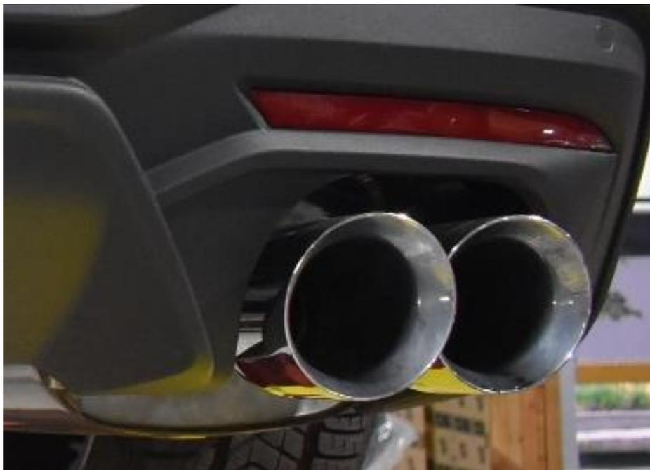
**Step 6: Check your exhaust system for proper clearance under the vehicle and also for tip alignment, tighten the clamps to 32-35 ft. lbs, checking tip alignment and clearances as you do. There should be a minimum gap of 25mm from the tips to the edge of the car, and the tips should be in 25mm from the outermost edge of the rear bumper.**
