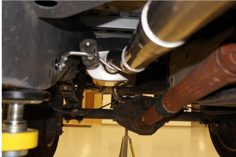
**Step 6:** Heat Shield installation. Drop the spare tire per the vehicle owner's manual instructions. Place the (2) J-nuts into the square holes on top of the cross-frame rail. Work the lip of the heat shield over the frame rail. Attach with (2) bolts provided. Using a 13mm socket torque to 20 N.m (15 ft-lb).
