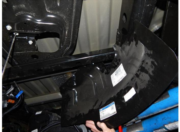
Using the band clamp provided, secure the side of the heat shield to the frame rail.
