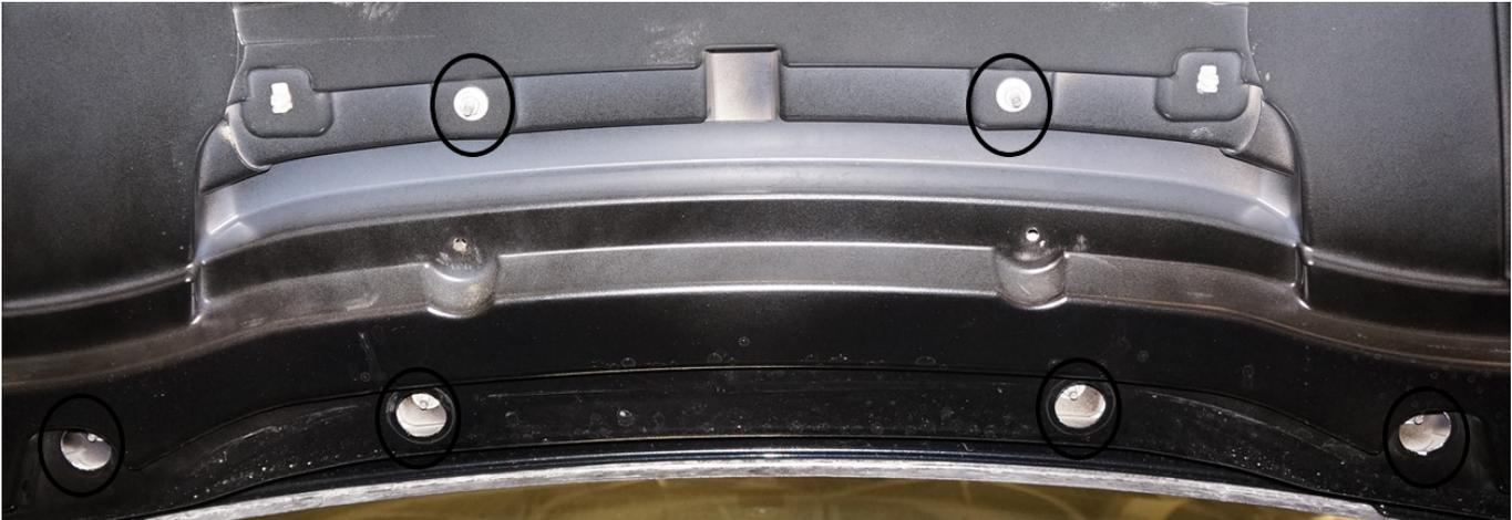
5. Compress retention clips where there is accessibility. Use non-marring tools to pry up the scoop starting from a back corner working around to the front and the opposite side.
