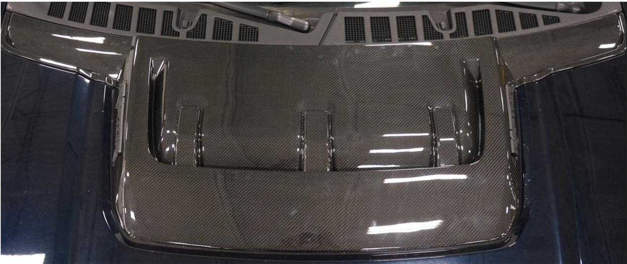
11. Install the supplied 6 Scoop nuts, original 4 nut covers and hood insulation.
