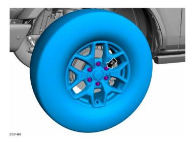
**Step 28:** Install the wheel nuts. For Bronco Raptor (M14 Wheel Stud), tighten to 200 Nm (147.5 lb-ft).
