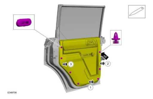
NOTICE: For re-installation, the tabs must be re-engaged to prevent the interior front door handle from becoming non-functional.
