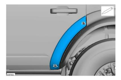
**Step 23:** Remove any tape remaining on the door by rolling off with thumbs.
