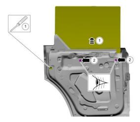
**Step 19:** Remove the rear door window glass.
