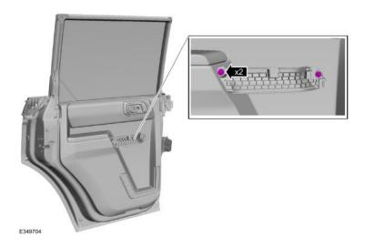
**Step 12:** Remove the rear door trim panel lower bolts. *Torque*: 36 lb.in (4.1 Nm)
