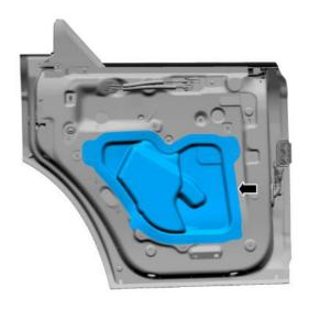
**Step 21:** Press the lugs from the interior of the door and release the retainers from the door.
