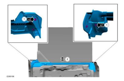
**Step 17:** Remove the rear door window glass adhesive covers.
