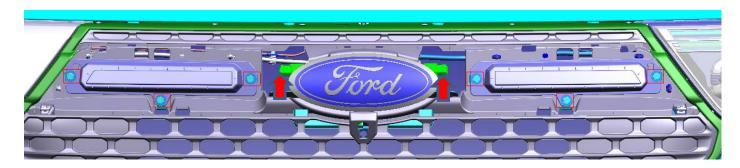
3. Plug light pigtail (not shown) into harnesses (x2). Hide the wirings behind light assemblies. Install aux lights into grille using the original fasteners. Torque 7.0+/-0.5 NM
