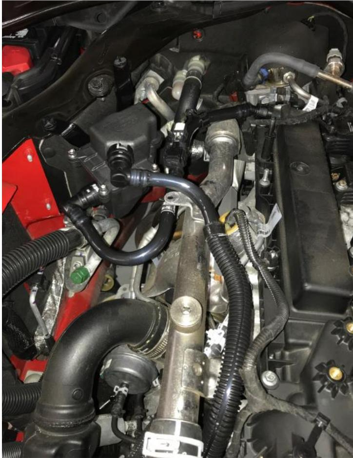
Step 4. Connect wiring harness to PCV tube sensor and reinstall engine cover.
