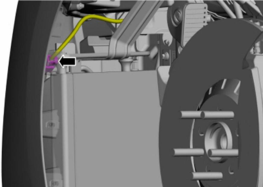
9. On both sides, remove the bolts, trim pin and separate the front bumper cover from the fender bracket
