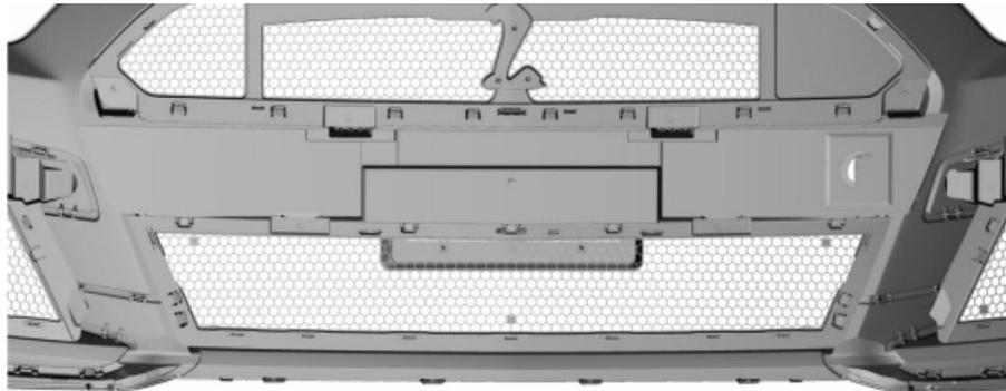
2. Remove the screws, release the tabs and remove the upper radiator grille panel
