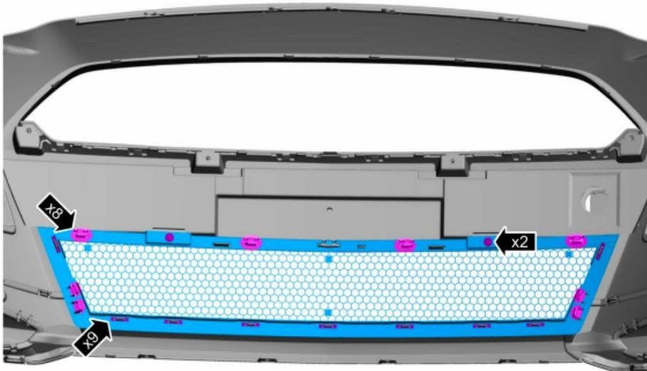
5. Release the tabs and remove the gloss black front bumper insert panel
