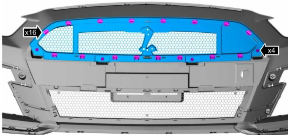
3. If equipped, remove the rivet blinds and the license plate bracket
