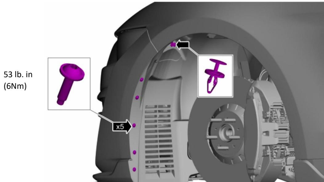
7. On both sides, remove push pins and position the fender liner aside
