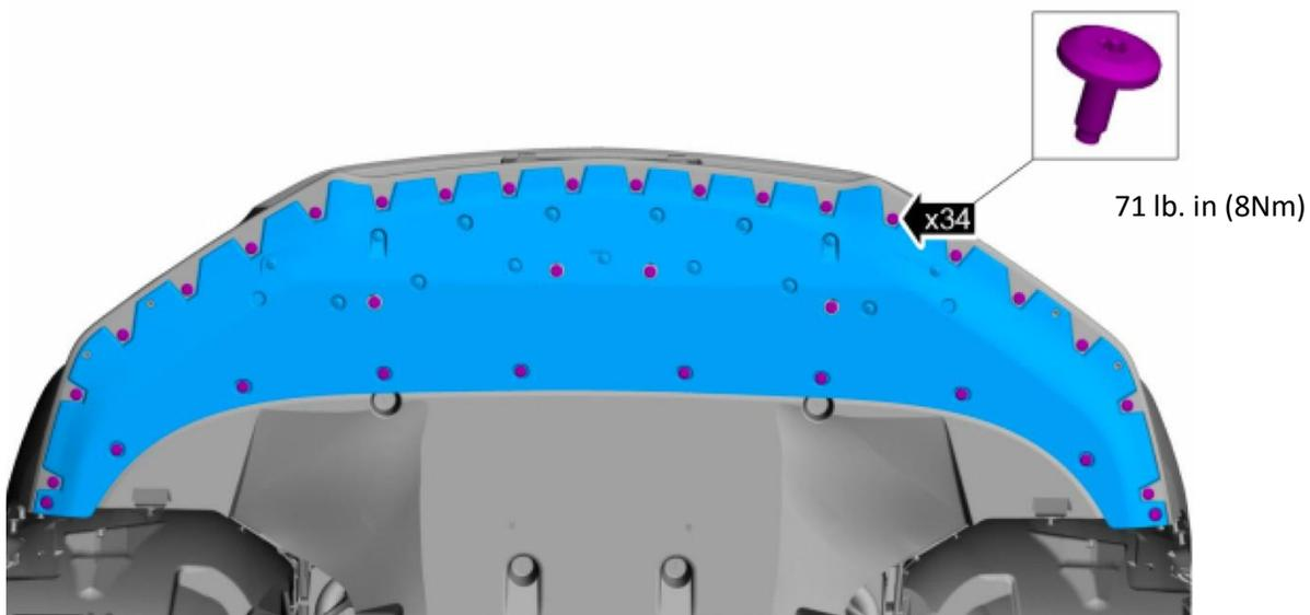
5. Remove the bolts, the screws, push pins, the trim pin and the under engine closeout panel
